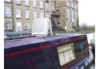
Figure 1. Boat with a SV collector (SolarVenti.UK)
