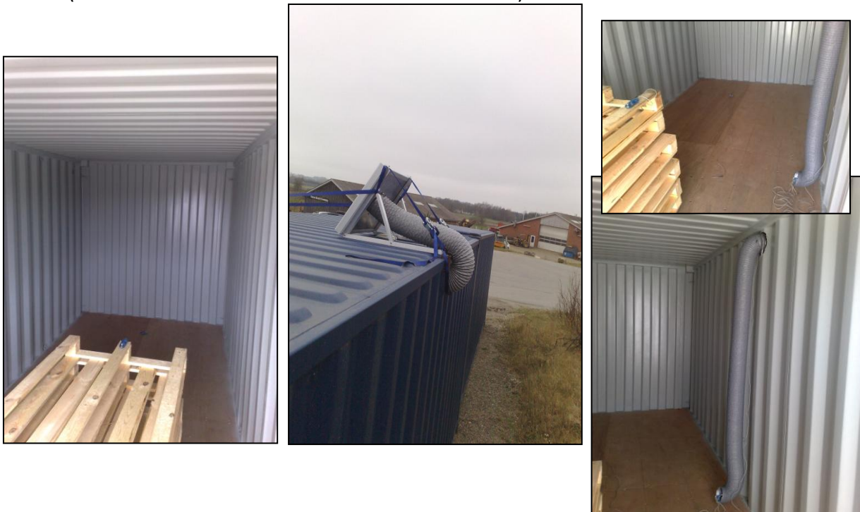
Figure 5. LEFT: control container CENTER/RIGTH: container with SolarVenti system
