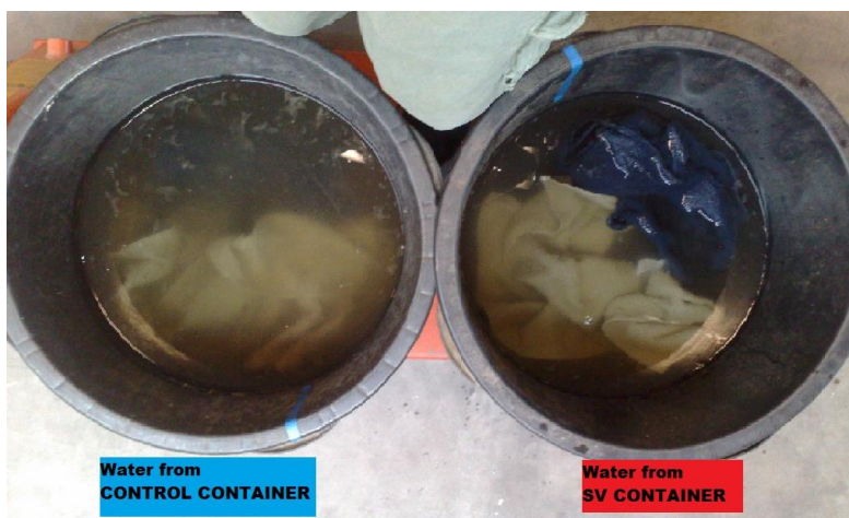
Figure 9: Water at the end of the test. The water from the control container is much corrupt and has a strong smell of black water.
